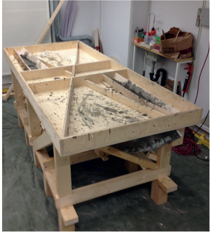
1 Reinforcement and foam border. 2 Inner shell connected with screws, waterproofed. 3 The formwork during casting.
