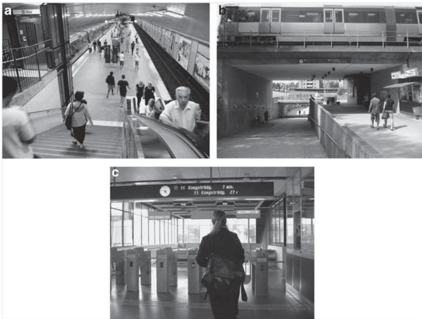
Figure 2: Environmental attributes of underground stations that promote security: (a) good overview of the whole station, clear sightlines of platforms in Odenplan station; (b) stations' external environment with clear overview from the train (and from outside) in Rågsved; (c) visible real-time train arrival display in lounge allows passengers better plan their trips in Akalla.
