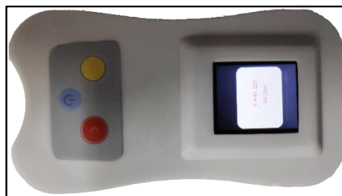
Figure 5. Developed optical reader for the quantification of the QDs fused sodium and potassium sensor films
