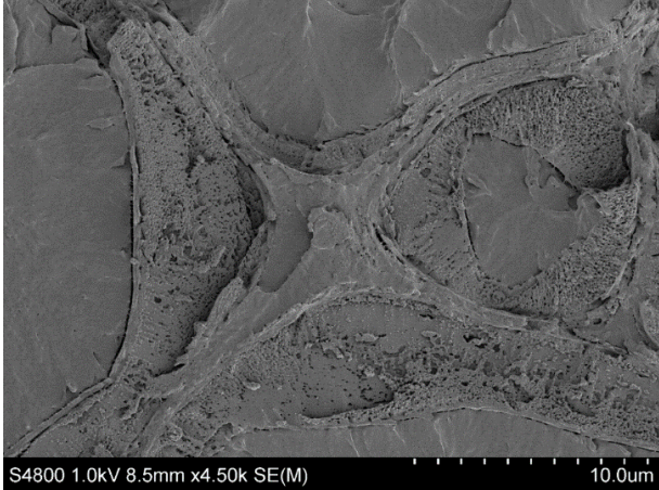
Fig. 1. Cross-sectional SEM image of a transparent wood sample revealing wood morphology and polymer filling cell lumens.
