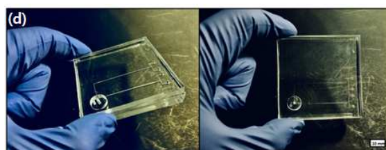
Figure 1. Fabrication of hierarchical structured microfluidic chip. (a) Fabrication of microfluidic channel. (b) Fabrication of floor channel. (c) Bonding process of the three fabricated channels by oxygen plasma treatment and heat curing. (d) Fabricated hierarchical structured microfluidic chip.
