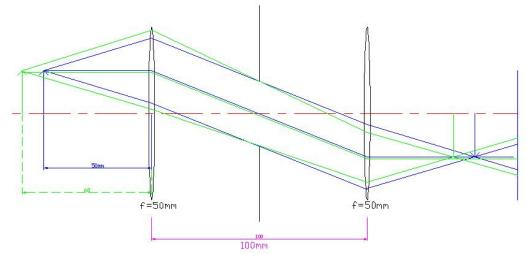
We have here two object positions, 50 mm and 60 mm in front of the first lens and we see that the displacements of the object and image are equal, since the lenses have equal focal length. The magnification is consequently equal to one.
